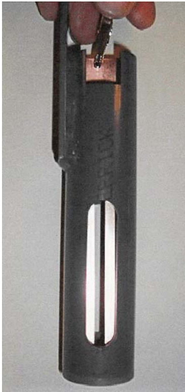
Figure 6. In – Site Plating Cell.
